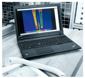
Infrared picture shows the temperature of a refrigerator handle 16 seconds after opening the mould. With carbon dioxide (right), the part cools down faster than with nitrogen (left).
